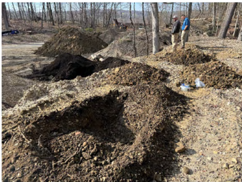
Photo 10: View of test pits conducted for sample collection in the berm.
