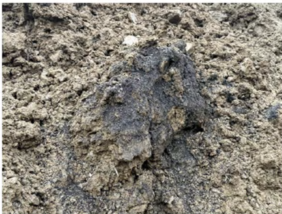
Photo 5: View of suspected asphalt millings encountered while segregating the soil into stockpiles.
